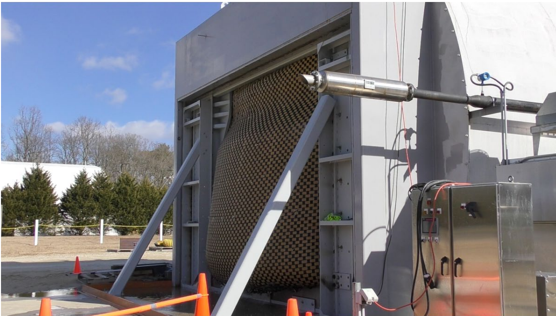
Portal flex gate undergoing water test at manufacturer
