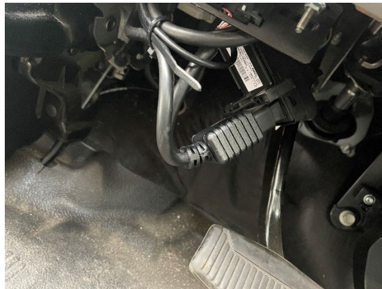
Photo 2: Showing the loose GPS device (black box with white sticker).
